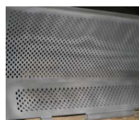
Screen protected against fine particle abrasion.
