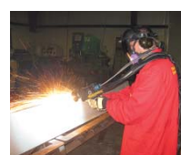
Protecting fan blades from abrasive wear.
